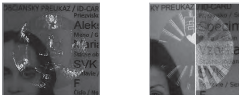
Figure 6 showing a) - counterfeit kinegram, b) - original kinegram
